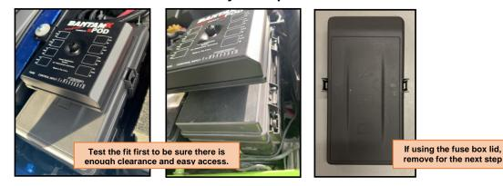
Cut the supplied template to the outer lines, locate a spot that will fit the 4 screw posts. Verify
