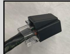
Be sure to keep protective cap on. Form a hook on the end of the fish line and wrap the connector with a little electrical tape.
