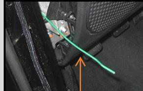
Run a fish line in from engine compartment
