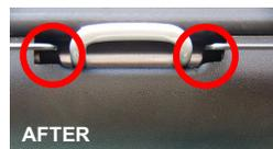
Trim about 1/2" wider and deeper as shown above on both sides to clear the bracket. Red lines show where to trim.
