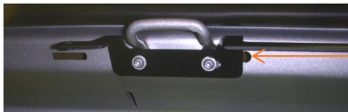
Keep this hole clear! It is used for the plastic windshield header alignment stud.
