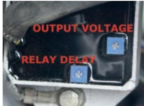
When mounted on the bike, the relay delay adjustment is on the bottom. The voltage adjustment is on the right. The adjustment procedure is as follows:
