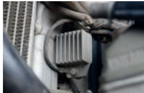
Install new RMSTATOR regulator using 8mm mounting bolt. Make sure attach black ground wire to mounting bolt. Orient with adjustment pots towards the bottom, so they are accessible. Route wires through frame, and plug in connector in OEM location.
