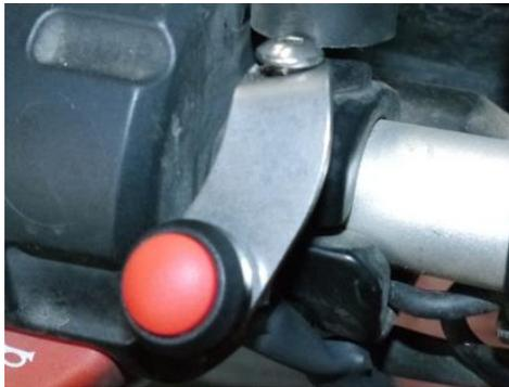
**Step 2.** Route the two toggle wires cleanly along your handlebars and behind your stock headlight. When completed plug the bullet connectors from the mode harness into the bullet connectors that coming off of the H4 connector.
