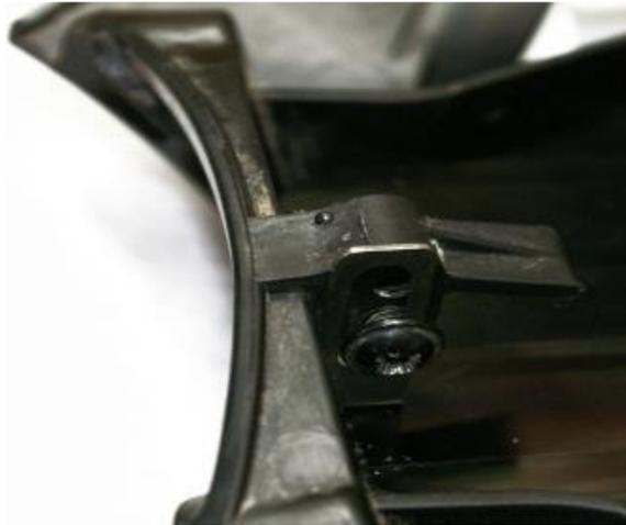
**For this step, you will utilize your stock headlamp adjustment screw. Note, the orientation of the screw does not matter. Simply insert the screw with a washer on both sides of the plastic ear, and tighten the nut.**
