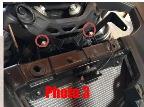
1. First start by removing the front panel that covers radiator. Pull gently and it should pop off.
