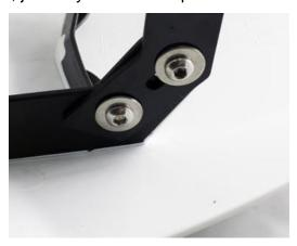
8. Install the provided long 6mm Allen head bolts, nylon spacers, washers, and Nyloc nuts as shown to the right.
