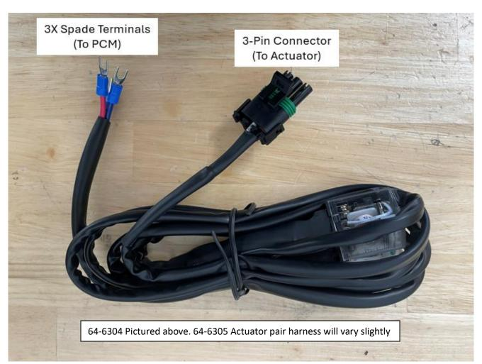
Connect the spade terminals to your power control module's (PCM) circuits following the chart below. For sPOD users, no modifications to the harness will be required. For other power management systems, the spade terminals may need to be cut off and replaced with a different terminal.
