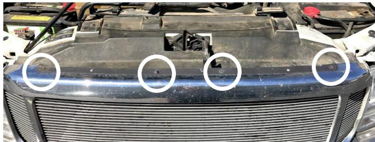
2. With a standard screwdriver (flathead), pry up on the four clips that hold the bottom of the grille on the vehicle. To access the clips, place the standard screwdriver in between the top surface of the bumper and under the grille. The photo below shows the location of the clips. The next photo shows the clip.
