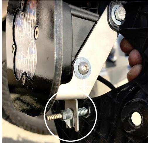
8. Adjust the housing bolts and OEM tilt adjuster until the desired fitment is attained.
