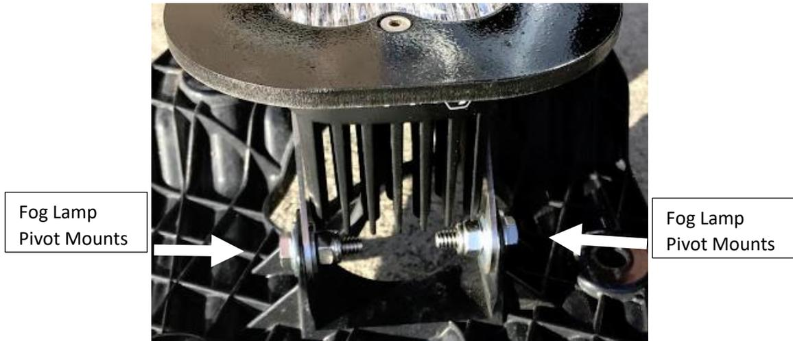
5. Reuse the OEM fog lamp bracket tilt adjustment hardware with the new bracket circled below.
