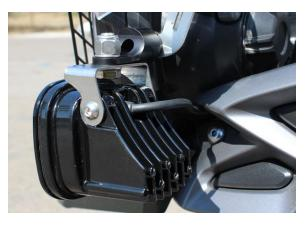
**Step 2:** Now that the mounting bolts have been installed and tightened you can begin mounting your Squadrons or S2 with a 3/8" socket and open-end wrench.
