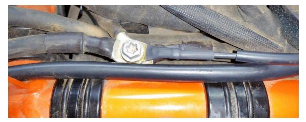
9.) Locate the accessory wire that is switched power via the ignition switch. In this case, it's a red wire with a black stripe. This wire can typically be found at the rear most part of the bike under the passenger seat by the taillight as shown in *Figure 15*.
