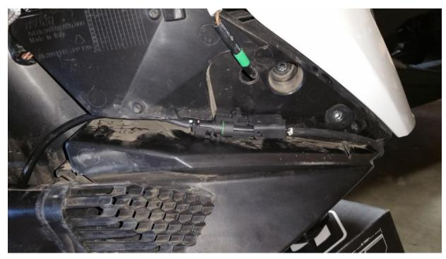
5.) Reattach plastic panels and mount lights using the supplied 5mm bolts, washers, serrated washers and spacers routing the wires beneath the spacer and behind the lights brackets as shown in *Figures 5, 6, 7 & 8.*
