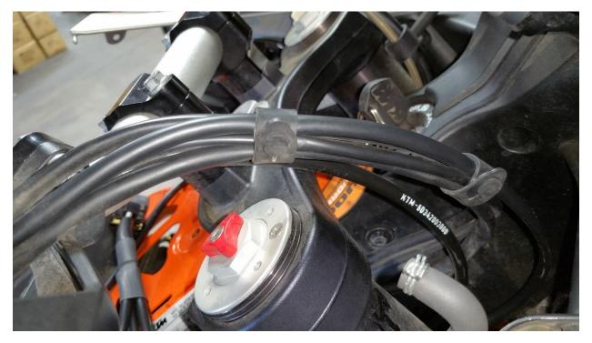
7.) With supplied 6mm bolt and short spacer, attach the switch to the handlebar clamp assembly as shown in *Figures 11 & 12*.
