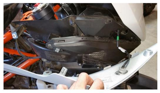
3.) Make a 5/16" notch in front portion beneath headlight with a Dremel tool or drill *Figure 3*.
