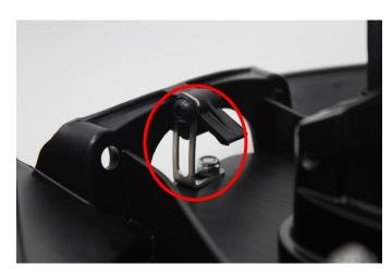
7. Using the provided black screw, install it in the hole that is closer to the back of the bike. To obtain full downward adjustment, you must trim the hole furthest from the chassis to allow the nyloc nut to clear. (Refer to circled area in figure 6)
