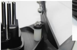
M5 Button Head Socket Cap Bolt and 5mm Nyloc nut as show in picture to
