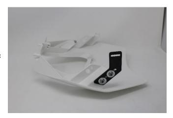
5. Slide the light into the housing lining it up the ears to bolt hole in the bezel. Put the spacer in between the ear and the light bezel. Insert the M6X40 with the washer from the front of the light, through the spacer and the ear, install the M4 nut. **NOTE:** Do not over tighten, you may risk cracking the plastic ear on the mask.
