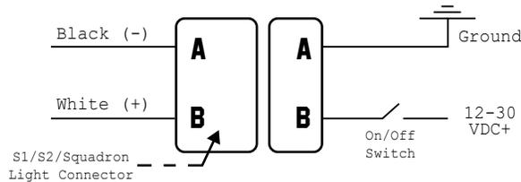
As with any electrical accessory, Baja Designs lights must have circuit protection (fuse or circuit breaker)
