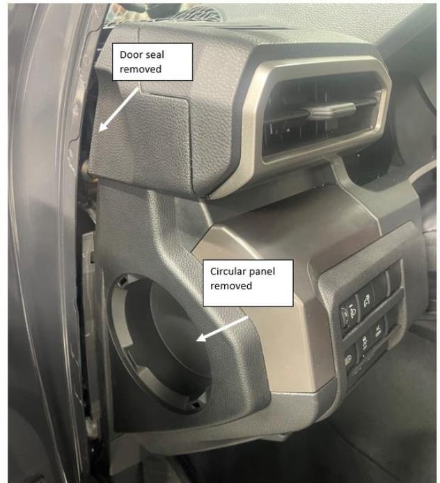
Remove the trim panel off the side of the dashboard by starting at the top edge and gently pulling away from the dash. Remove the chrome trim panel by pulling parallel to the arrows pictured.
