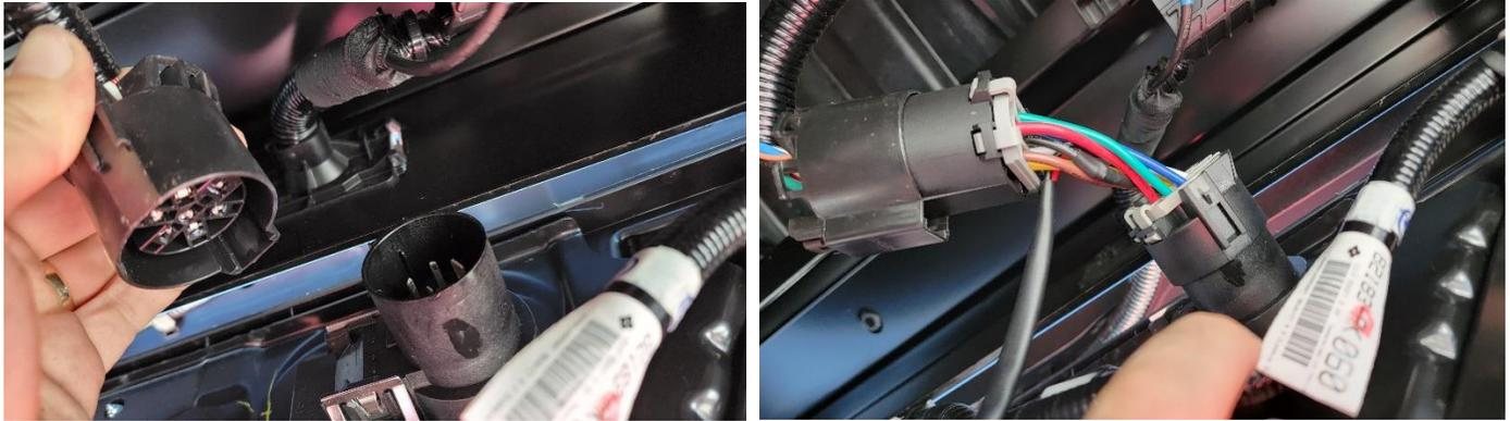
**Step 7 Toggle Only:** Remove the protective cap from the connector at the rear frame powered circuits junction box of the vehicle (A) -> (B). The junction box is located underneath the vehicle near the rear left (drivers' side) taillight. Connect the Rear Circuit Output Adapter (60-0103) to the Splitter harness installed in step 6 and to the OEM Junction Box (C). Tie all loose wiring neatly away from hot, rotating or sharp components using the provided Zip-Ties (20-1612).
