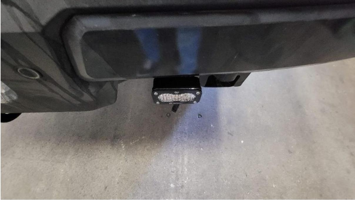
**Step 6:** With the lights secured in place, connect the Universal Harness Splitter 55" (61-3606) to both lights. Ensure the shorter side of the splitter goes to the left (drivers' side) light.
