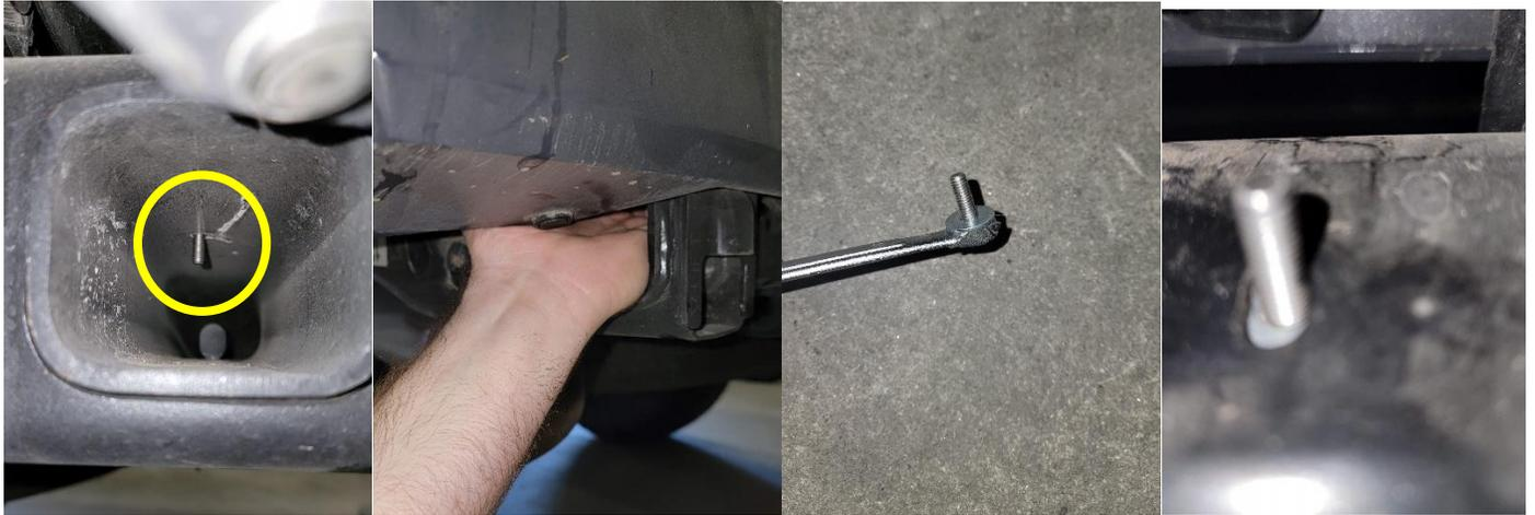
^Screw depicted above is for locating demonstration. For installation, insert screw from inside tube.
