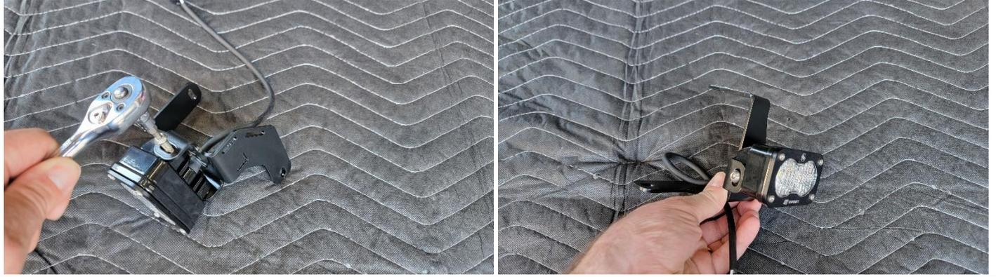
**Step 2:** Place a M6 Hex Screw (20-1243) and a M6 Washer (20-1141) inside both lift point frame hole going through the inside hole with the threads facing down. Align the Reverse Bracket (Left = 44-7684 and Right = 44-7685) bottom mounting holes (near the letter identifier) with the screw and secure it to the frame with a M6 Washer (20-1141) and M6 Locknut (20-1690). Loosely tighten the nut so that the top mounting point can be adjusted if necessary.
