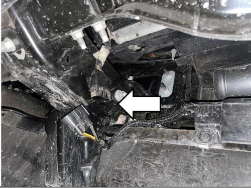
**Step 11:** Remove the 2X bolts connecting the bumper to the bumper support using a 15mm socket.
