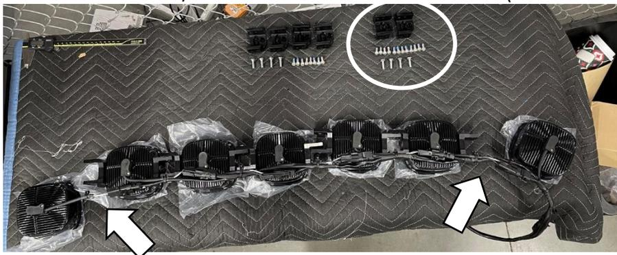
**Step 3:** Split the linkable in between the 4<sup>th</sup> and 5<sup>th</sup> light. Remove the link on the 4<sup>th</sup> light using a 3/16" & 5/32" hex bit.
