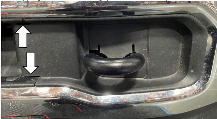
**Step 13:** Free the rubber trim from the OEM fastener (E) by using a trim removal tool to loosen the fastener and pry the rubber trim out from behind it. (Repeat steps 11-13 on both sides)
