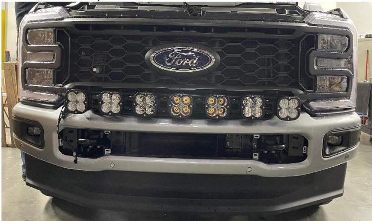
**Step 22:** Tuck the linkable connector lead away into the bumper and make sure it drops down behind the passenger side fog light.
