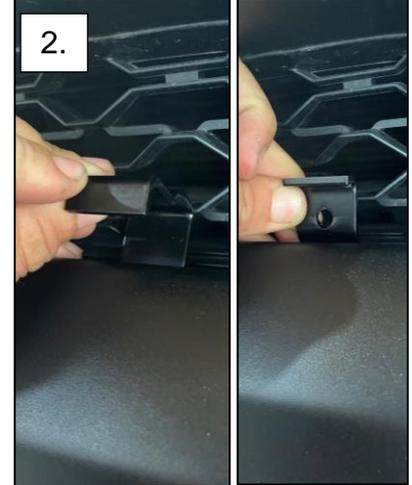
3. Fasten the S8 bracket onto the two clasping brackets. Use a 7/16" wrench and socket to fasten down the bracket. Do not completely tighten down, allow the bracket to be re-positioned on the bumper.
