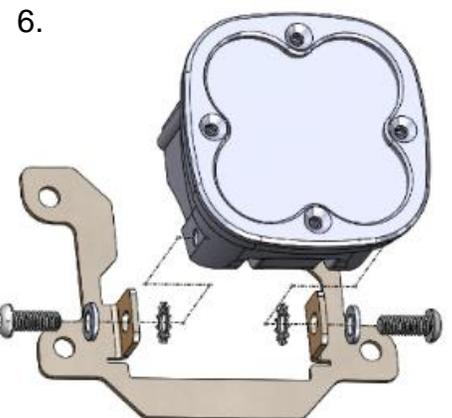
Re-torque all the fasteners after 100 miles.
