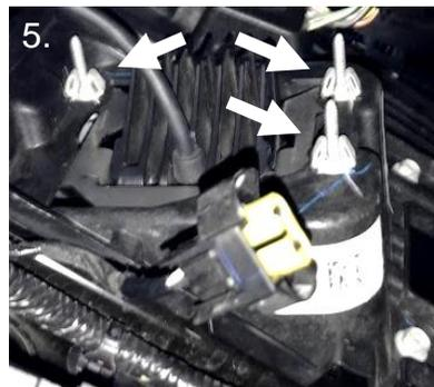
\*\* Image shows the screws from behind with fog bracket still installed.
