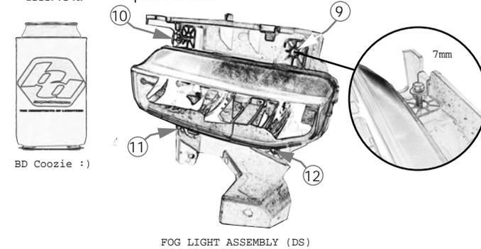
5. Mount the S2's with hardware as shown below. The S2 closest to the engine should be mounted ~35/64" away from the nearest edge of the bracket. The other S2 should be mounted ~53/64" away from the nearest edge. Using the 7mm socket, with extension, and the OEM hardware attach the Baja Designs bracket to the OEM plastic bracket in all available mounting locations.
