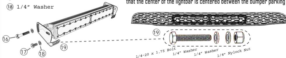
3. Attach the bracket to light bar as shown to the left. Then, replace the OEM bumper bolts with the hardware shown in region (19). Finally, adjust the bar so that the center of the lightbar is centered between the bumper parking sensors.
