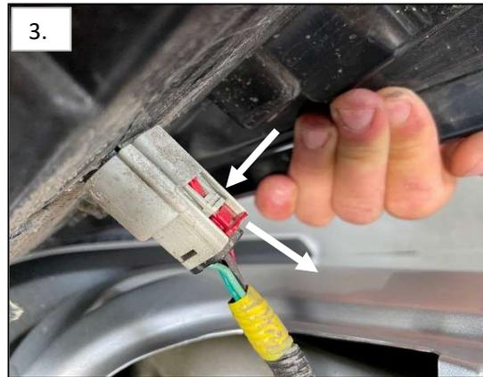
**4.** Locate the reverse light power wire. It will be the light green wire located on the bottom right of the connector.
