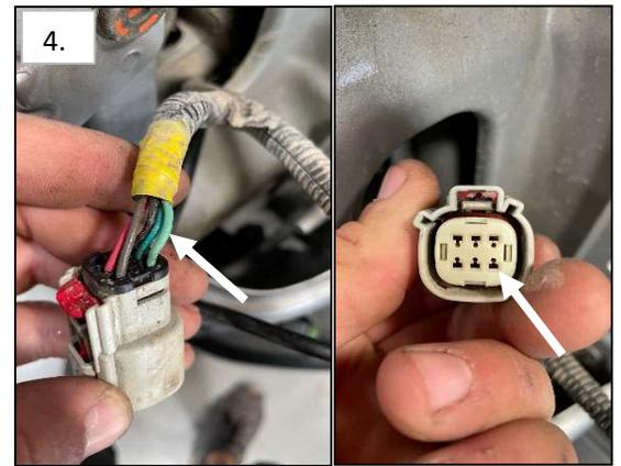
**5.** Use the splice connector on the reverse light harness and clasp the two ends together over the light green power wire.
