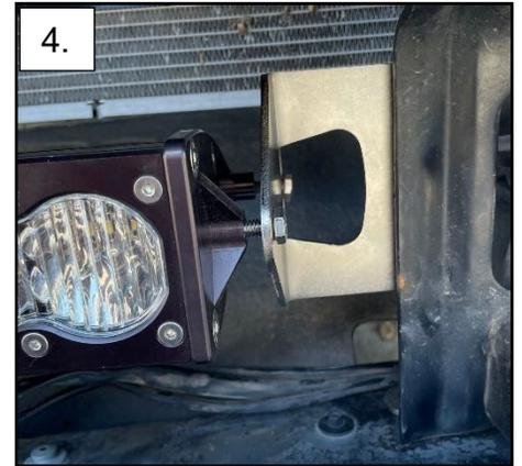
5. Adjust the light bar by Rotating until the desired lighting angle is achieved. Using the 7/16" wrench and socket torque down the bolts to 4 ft-lbs.
