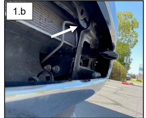
2. Install the bracket as shown using the 2x bolts removed from step 1. Leave bolts loose.
