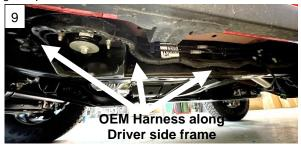
10. The main harness (upfitter or toggle switch) will need to be unraveled. Route the light lead of the harness down the driver side firewall away from any hot, sharp, and/or rotating components. Continue routing the harness until it reaches the 10ft extension. Connect the main harness lead to the extension. Remove the slack and tie the harness as needed, pulling up into the engine compartment. Any extra harness length can be tied up and placed into the inner driver side fender.
