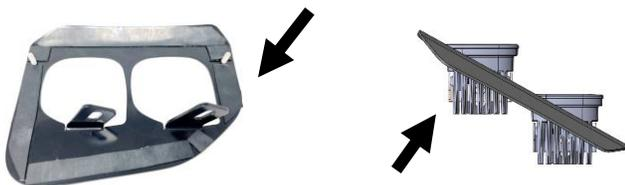
8. Mount each squadron onto the Baja Designs fog bracket in the desired configuration using the 9/16" wrench and socket. Mount it onto the bumper from the outside and hand thread on the washers and nuts. Carefully adjust the bracket to sit nicely in the bumper contours and then gently tighten the nuts with the 10mm wrench. **Do not over tighten as the studs can pull through.**
