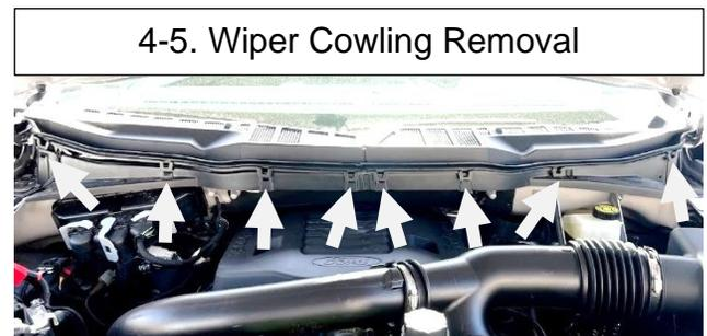
6. Once the cowling is loose and all the clips have been undone, carefully pull the driver side cowling up (axially) around the wiper arm hub. Take special note of the windshield wiper fluid hose attachment points for installation later. Repeat for the passenger side. Place both wiper cowling panels on top of the engine for the moment.
