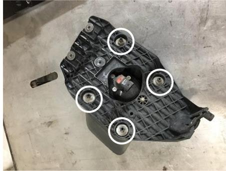
4. Using the 3mm Allen wrench, remove the four Bezel bolts (circled below) that hold on the standard Squadron bezel. Replace the bezel with the provided Super Duty bezel and retighten hardware. With the 4mm Allen wrench, screw in the Squadron housing bolts through the washer, bracket, serrated washer, and then into the light housing. Repeat for the opposite side of the housing.
