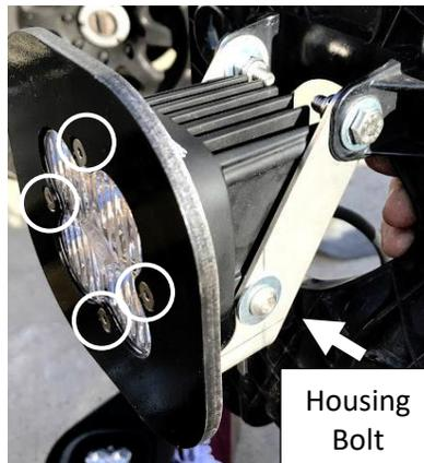
5. Using the  $\frac{7}{16}$ " wrench and socket wrench, tighten the  $\frac{1}{4}$ " bolt into the washer, plastic bracket, steel bracket, washer, and nylon locking nut. Repeat for the adjacent fastener.
