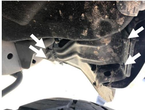
2. Unplug the OEM fog light connector from the harness. With the 8mm socket wrench, remove the three bolts holding on the fog light assembly circled below. Carefully remove the assembly from the vehicle. Repeat for the driver's side.
