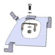
2. This kit places each Squadron light upside down inside the fog pocket. Using the 2.5mm Allen wrench, remove the four bezel bolts on the face of the light. Remove and spin the bezel and lense 180 degrees, then reinstall. Assemble the light onto the bracket with the rest of the hardware in the parts bag (see exploded view below). Tighten lightly for adjustment later. Repeat steps 1 and 2 for the opposite side light and bracket assembly.
