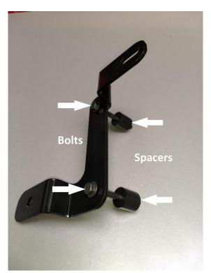
Step 3: Install driver and passenger side brackets onto their corresponding sides and tighten snugly.
