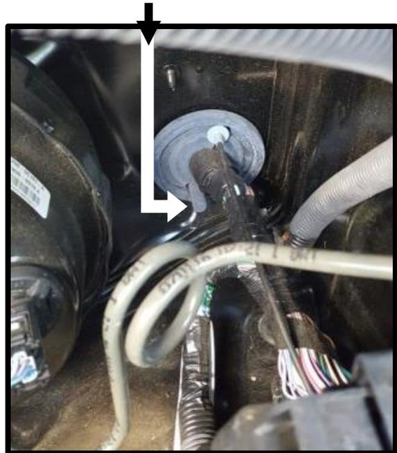
20. Place the bumper cover back onto the vehicle and install the top center plastic fastener. Use the 10mm wrench to replace the two nuts from step 8. Replace the radiator shroud and wiring clip from step 19. Then use the 10mm socket to replace the nuts from step 7 and bolts from steps 6-4.
