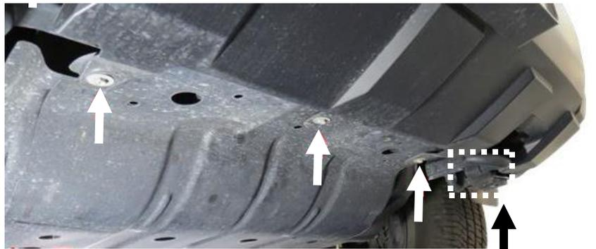
7. With the 10mm socket wrench, remove the two nuts on the bottom corners of the bumper cover (one per corner). Carefully push the bumper forward enough to free the stud (See passenger side image on right with fastener circled).
