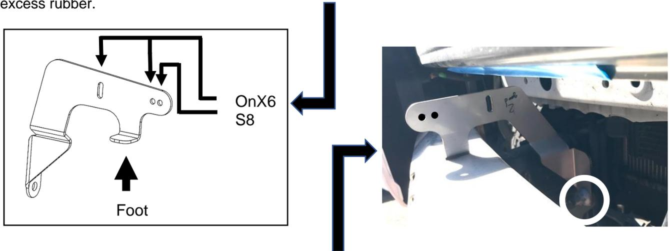
13. Take the bracket labeled "PS" and place it over the single stud circled above on the right. Repeat on opposite side with the "DS" bracket. Thread each nut onto the studs until hand tight.
