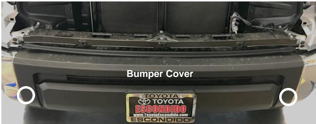
Carefully pull down the bottom edge of the bumper cover so you can access behind the circled fasteners shown above. With the 10mm wrench, reach into the back of the bumper near the bottom left or right and carefully loosen the nut. It should easily come off by hand after breaking loose with the wrench. Repeat for the opposite side. (Passenger side nut arrowed in image next to step 7)
