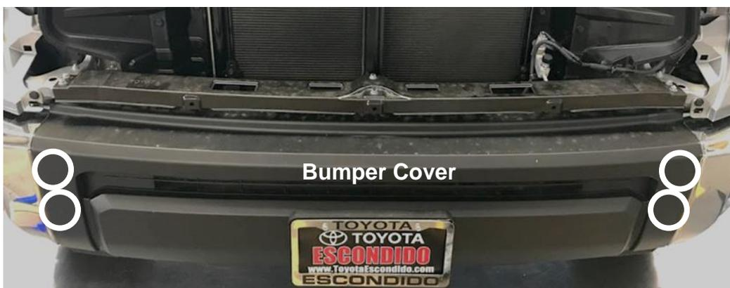
10. With the Flathead screwdriver, pry up the plastic fastener on the center of the bumper cover and remove. Now the bumper can be lifted and removed. Place the cover on a soft surface.
