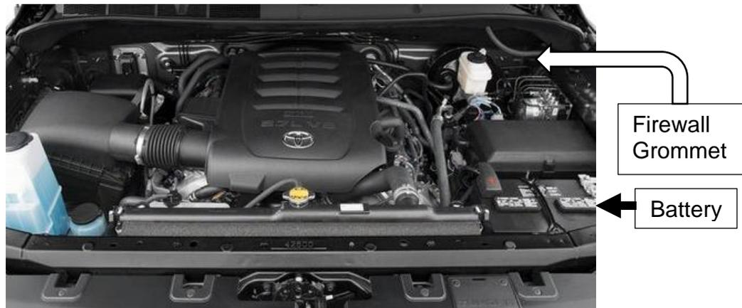
17. Label all switch terminals and their locations. Remove terminals from switches. Locate the driver side wiring passthrough grommet (see image below). Cut through the nipple at the bottom of the grommet. Use Vaseline, or lubricant to help pass the wires through. Pull the necessary length through the grommet to reach the dash mounting location. Reattach the terminals and mount the switch. Tie all wires away from any hot and/or rotating components.
