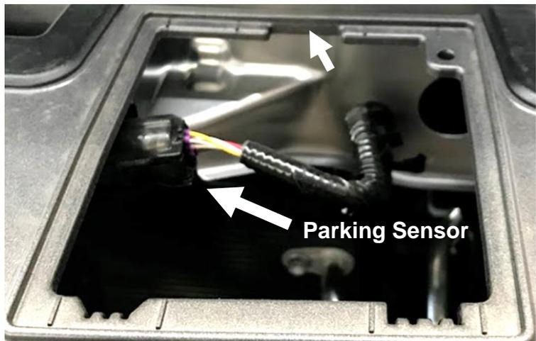
3. To remove the grille, carefully pull the bottom corner with constant force until it unclips. Repeat for the other corner. Then, lift at the top of the grille to remove and place it on a soft surface.
