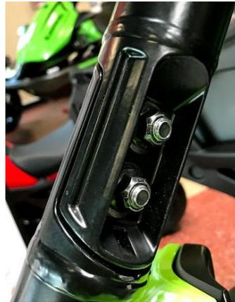
2. Locate the new A-Pillar brackets, bolts, spacers, washers, and nuts. The driver side assembly is shown below. Use the picture for reference to identify the driver side bracket. If the cage shifted after step one, it may be necessary to push the cage inward to realign the mounting holes.
