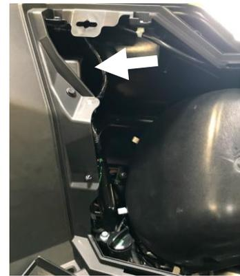
2. Remove the in-cabin rear access panel by pulling the top edge toward the front of the vehicle (see image on next page). The picture on the right below shows where the A-pillar light switch leads can be routed. The switch can be removed to route wires through and then reattached. Take note of switch terminal configurations.
