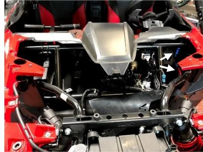
17. Unravel the harness. Attach the wiring harness ring terminals to the corresponding battery ring terminals from step 2 using the provided 7/16". Place provided shrink tubing over each connection and carefully heat until insulated. Tie safely out of the way of hot/rotating components.
