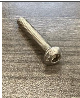
(20-0084) (Qty: 6) M6-1.0 35mm Length Button Head Hex Drive Screw
