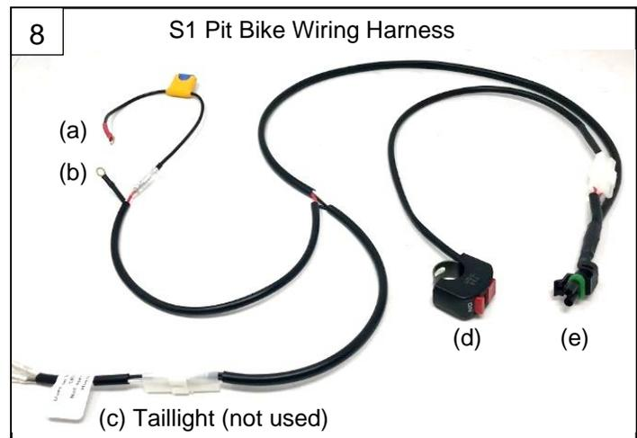
8. Connect the harness light plug (e) to the light power cord and route the handlebar switch (d) to a suitable location on the handlebars. Use a Phillip's head screwdriver to mount the switch. Route the battery leads (a,b) back to the battery along the frame along the existing OEM wiring harness.
