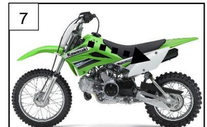
7. Remove the seat and the gas tank (models vary). Unravel the provided S1 Pit bike Moto Kit wiring harness and locate the light plug lead.
