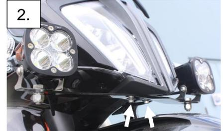
3. Assemble both the lights with the associated hardware using the exploded images for reference. Notice the S1/Squadron bracket orientation. Mount both lights to the bracket shown in step 2.
