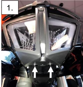
2. Use the 4mm Allen wrench to mount the BD Squadron/S1 KTM 790 bracket to the headlight with the provided bolts and washers.
