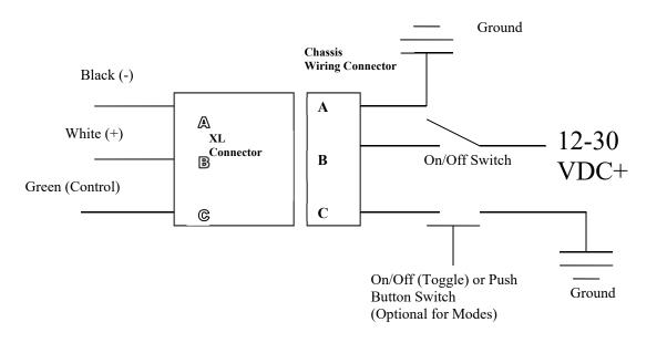
When using the optional On/Off (Toggle) or Push Button Switch, depressing the switch will dim the light 20% from 100% power. Depressing the switch again will toggle back to full power.
