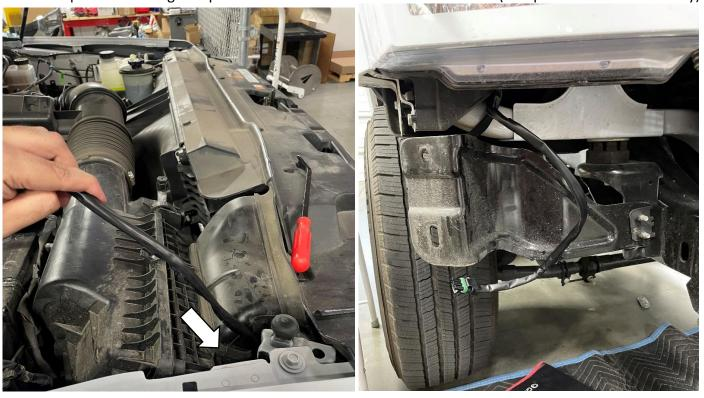
**Upfitter Only** Locate and detach the upfitter fuse box located near the PS fuse box (boxed) by pressing in the two locking tabs (1&2) and lifting up to access the bundle of wires underneath it. Take the included upfitter wiring harness and attach the white wire scotchlok (I) to the desired auxiliary wire using a set of pliers. Reinstall the upfitter fuse box. Attach the connector on the upfitter harness to the XL Linkable connector.
