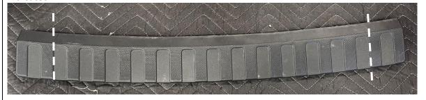
**Step 18:** Loosely install your pre-assembled XL Linkable from Step 8. Install 4X M8 Socket head screws, 4X M8 nyloc nuts and 8X M8 Washers using a 13mm wrench and a size 6 Hex bit.
