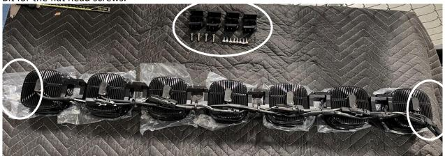
**Step 2:** Remove 2X links from the inside edge of the outermost lights using a 3/16" hex bit for the socket head screws and a 5/32" hex bit for the flat head screws (None of these flatheads will be reused).
