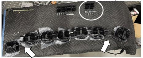
**Step 3:** Split the linkable in between the  $4^{th}$  and  $5^{th}$  light. Remove the link on the  $4^{th}$  light using a 3/16" & 5/32" hex bit.
