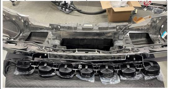
**Step 20:** Tighten the mounting bolts for your XL Linkable. Manually lift your XL Linkable from the center and tighten the 2X bolts (H) securing your pre-load assembly from Step 5.
