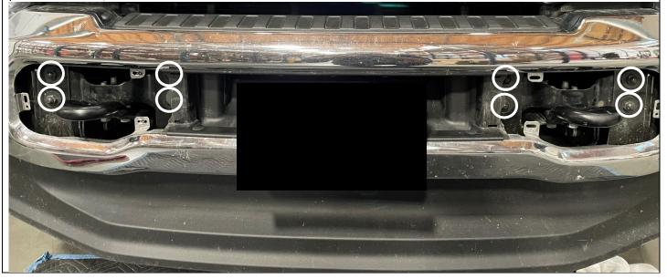
**Step 17:** Remove the plastic trim panel on top of the bumper. Use pliers to squeeze the clips from the inside and push them out. Remove any clips tying the panel to the harness. Cut the trim panel at the lines indicated.
