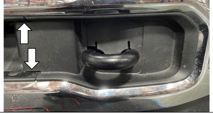
**Step 13:** Free the rubber trim from the OEM fastener (E) by using a trim removal tool to loosen the fastener and pry the rubber trim out from behind it. (Repeat steps 11-13 on both sides)
