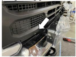
**Step 23:** Make sure no harnesses are being pinched. Make sure your bumper is level then fully tighten down the bumper. Reinstall all trim panels and bolts removed from steps 10-17. Make sure the OEM electrical connectors are reinstalled and the adaptive cruise bracket is reconnected.
