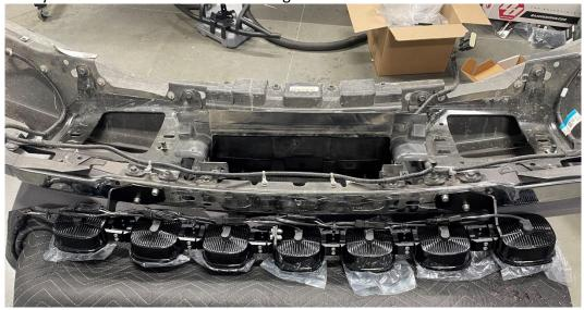
**Step 19:** Loosely mock-up your large trim panel underneath the XL linkable. Note how much more material needs to be trimmed from the sides to fit around the mounting brackets. Trim the panel to fit (Should look roughly as pictured below). Lift the loose pre-load assembly and install your trim piece underneath.
