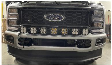
**Step 22:** Tuck the linkable connector lead away into the bumper and make sure it drops down behind the passenger side fog light.
