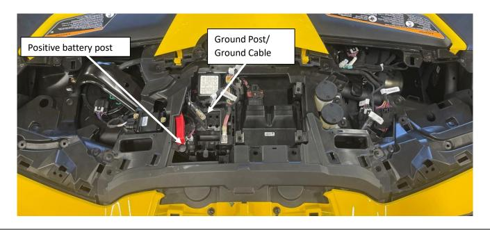
**Step 24:** Re-install all trim panels by following steps 2-6 in reverse. Make sure the harness is secured under the hood/ trim panels.
