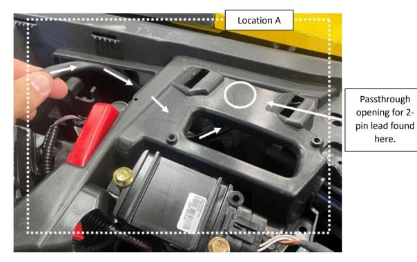
**Step 15:** Install connector onto exposed pins \*Critical\*
