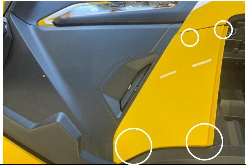
**Step 6: U**sing a 10mm socket and T27 Bit/Driver remove 4X Bolts. Remove passenger trim panel C.
