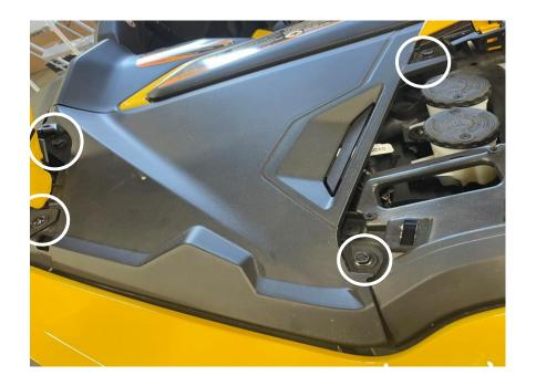
**Step 7:** Use 9/16" wrench and socket to mount the S2s on the bracket (44-9414) provided. Tighten the light on it's maximum forward bend angle for ease of installation and better field of view.
