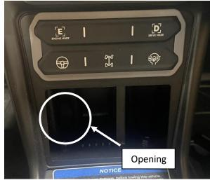
**Step 20:** Remove the blank from the switch panel.
