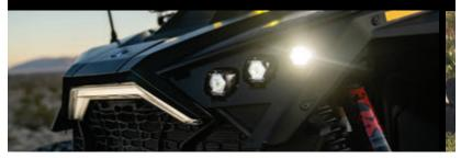
Designed from the ground up, the S1 combines a specialized reflector and LED making it highly adaptable for applications that need light in a small package.
