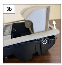
4. With the flathead screwdriver, press in on the sunglass holder pivot (circled in step 3b) and pull on the side wall until it is free. Twist the holder until it can be removed. Place aside, it will not be reused.
