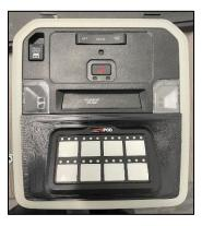
9. Route the small ethernet cable through the hole from step 6 and plug it into the Tundra sPOD switch panel assembly. With the provided socket head hardware, washers, and 3mm Allen wrench, tighten the assembly into the console through the holes from step 5 (arrowed).
