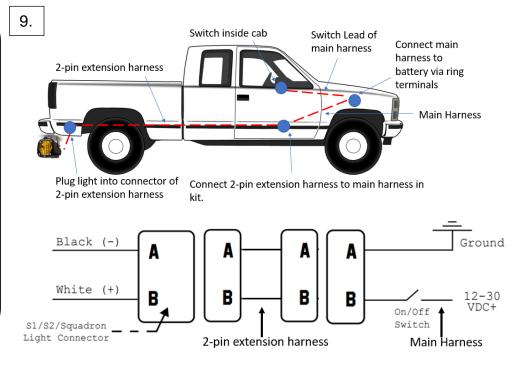
10. Now, plug in the Baja Designs S1 plug into the included wiring harness lead. Zip tie all wires so that they do not interfere with any objects and can't break free. The light should turn on when the vehicle is on and in reverse if you purchased 44-8153, otherwise if you purchased 44-8157 then the light should turn on when the vehicle is on and the toggle switch is on.
