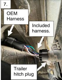
8. NOTE\* - Some vehicles have a plastic ring around the connector that prevents the included reverse harness from seating correctly. If you don't hear or feel a "click" when mating the harness to the connector, simply grab some pliers and pull the extra connector component off the stock connector. This piece is especially apparent on Ford vehicles.
