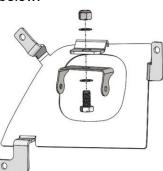
2. This kit places each Squadron light upside down inside the fog pocket. Using the 2.5mm Allen wrench, remove the four bezel bolts on the face of the light. Remove and spin the bezel and lense 180 degrees, then reinstall. Assemble the light onto the bracket with the rest of the hardware in the parts bag (see exploded view below). Tighten lightly for adjustment later. Repeat steps 1 and 2 for the opposite side light and bracket assembly.
