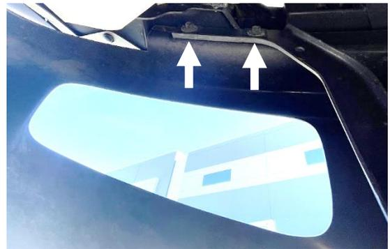
**Step 2:** Once that has been done, you can begin installing the Baja Designs Fog Pocket Mounts with the provided 8x45 Bolts. Use provided spacers in-between the brackets and the mounting surface as shown. Repeat for both sides. Driver side bracket shown.
