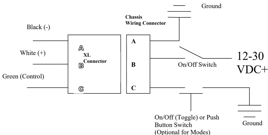
When using the optional On/Off (Toggle) or Push Button Switch, depressing the switch will dim the light to 50% power. Depressing the switch again will toggle back to full power.
