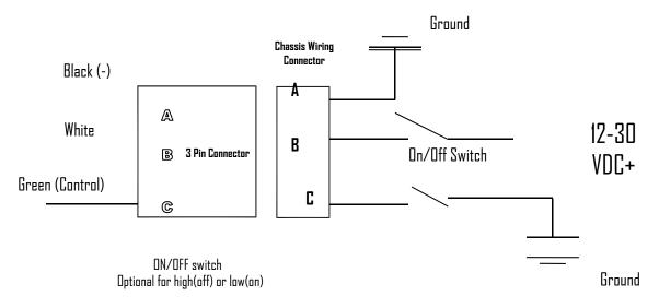
When using the 2<sup>nd</sup> Switch, the light will dim to 75% power. Turning the switch off will toggle back to full power. This is to be used when your vehicles charging system cannot produce the necessary voltage (13.5V or higher) to keep the vehicle charging. Included with your light is an inline "Hi-Low" adapter in case you **DD NDT** want to wire a secondary "On/Off" switch.
