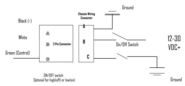
When using the 2<sup>nd</sup> Switch, the light will dim to 75% power. Turning the switch off will toggle back to full power. This is to be used when your vehicles charging system cannot produce the necessary voltage (13.5V or higher) to keep the vehicle charging. Included with your light is an inline "Hi-Low" adapter in case you **DD NOT** want to wire a secondary "On/Off" switch.
