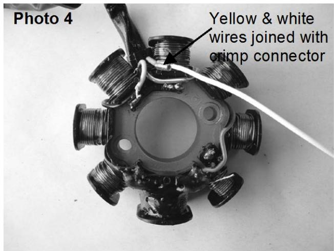
to the yellow wire from the stator as shown in Photo 4. Solder this connection after it has been made.
