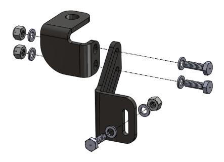
3. Using the provided ½" hardware, bolt in the brackets to their corresponding mounting locations. As can be seen below, take care to avoid scratching the roll cage by using plastic, masking tape, a rag, etc.
